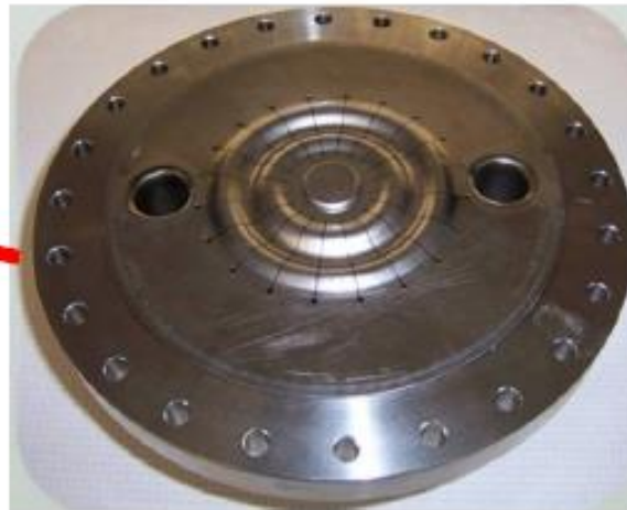
Niobium push-pull tuning plate with convolutions and cuts
