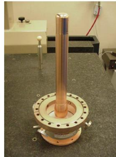
SNS coupler based on KEKB design
