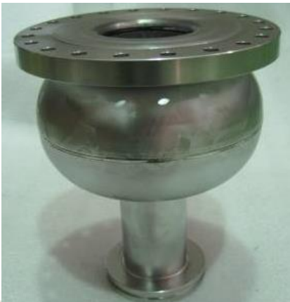
Single cell cavity
